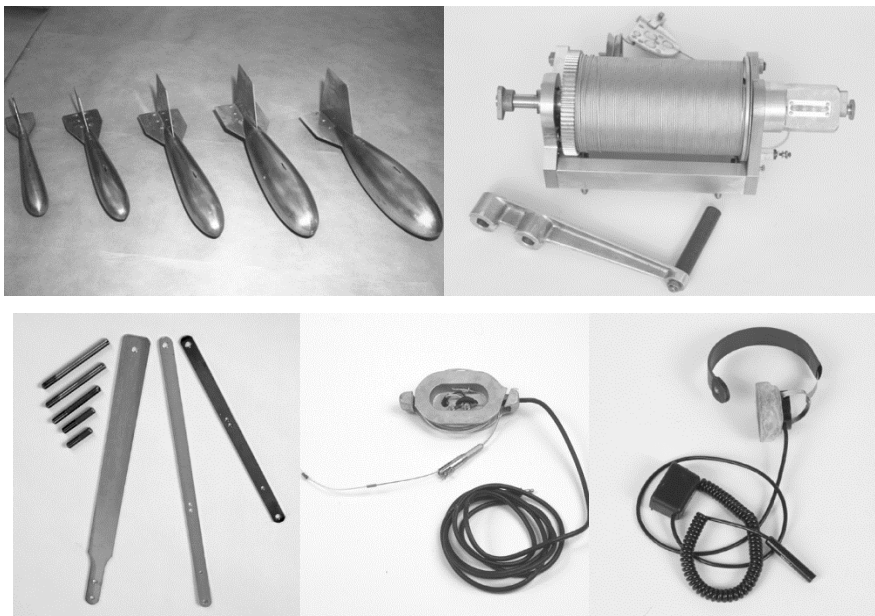
(a.重錘；b.吊桿及插梢；c.捲揚器；d.懸索；e.耳機)
