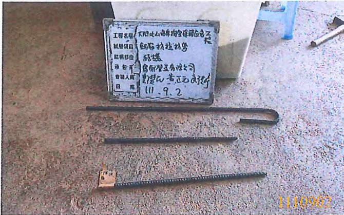
SD280W D13 鋼筋取樣試驗
