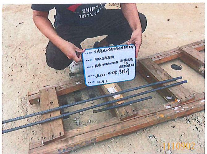
SD280W D13 鋼筋取樣
