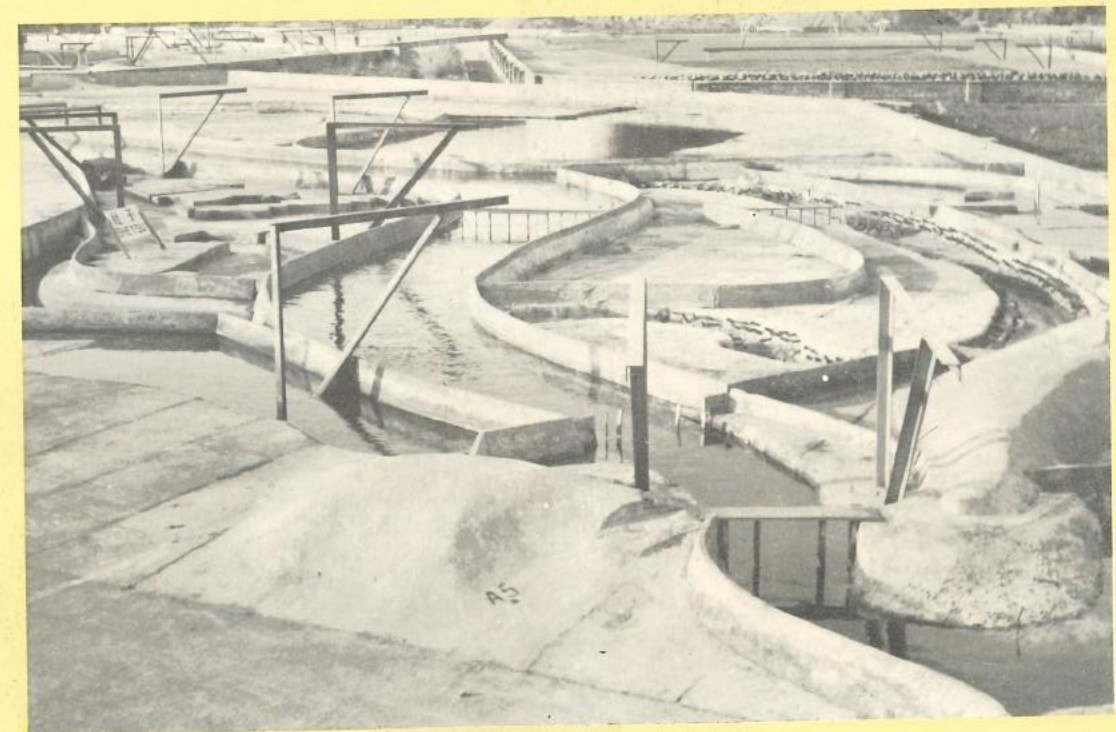
基隆河新河道模型及實驗情形 Hydraulic model test for the project of the new channel construction of Kee-Lung River.
